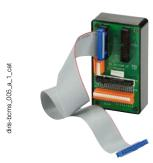
During installation and connection of the panel it is possible that damage may occur to a CT on a 6 or 9 CT strip. This kit enables any damaged CT to be replaced, avoiding the need to replace the entire CT strip. Any CT can be replaced without disconnecting cables or shutting down the installation.
