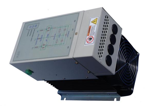
ABB's pF-TSM is a Thyristor Switch specifically designed for high speed switching of Power Factor Correction Capacitor Banks. (10kVAr, 25kVAr & 50kVAr @ 415/440VAC, 50Hz).
